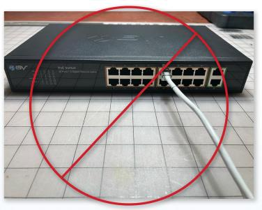
When connecting to the router use the uplink ports, not the standard PoE ports
