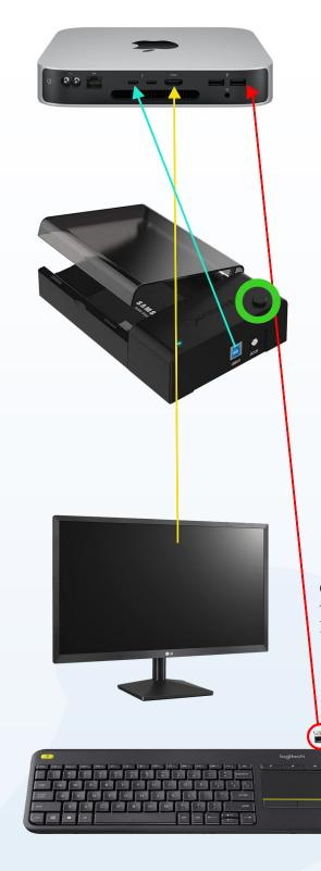
The Sabrent hard drive enclosure(s) will connect to the server with the cable that came in the package (USB-B to USB-C cable) (Illustrated with the teal line). The drive needs external power, AND the power button (Green circle) turned on to fully function.
